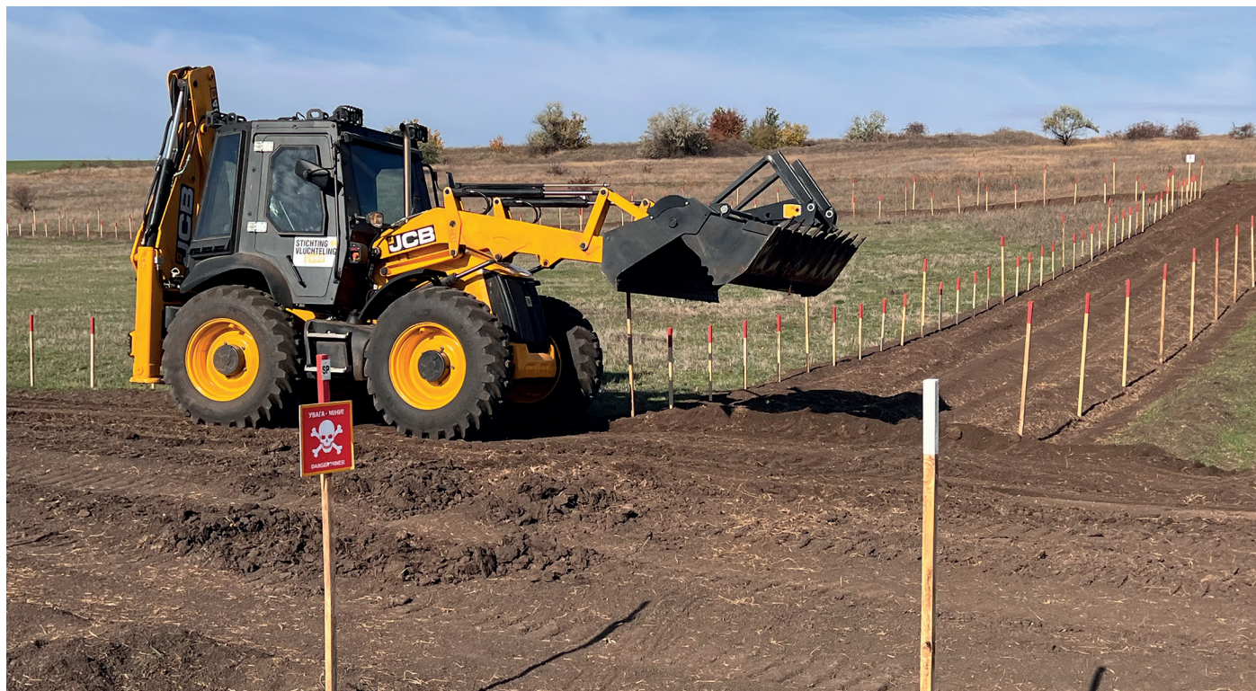
Figure 12: Armoured JCB vehicle clearing access routes. Mykolaiv Oblast, Ukraine
