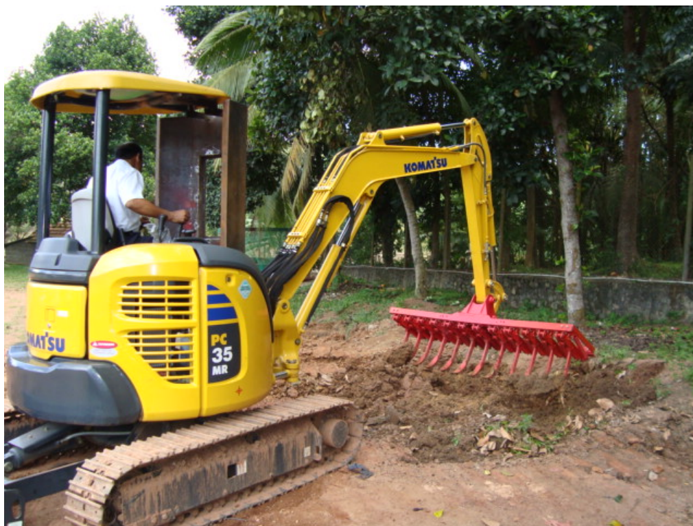
Final modification and testing of 4 new excavators with rake attachment is currently ongoing prior to field deployment at the beginning of October
