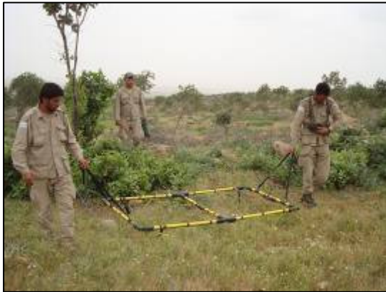
MAG MAT team conducting clearance operations in Dohuk using Large Loop detector
