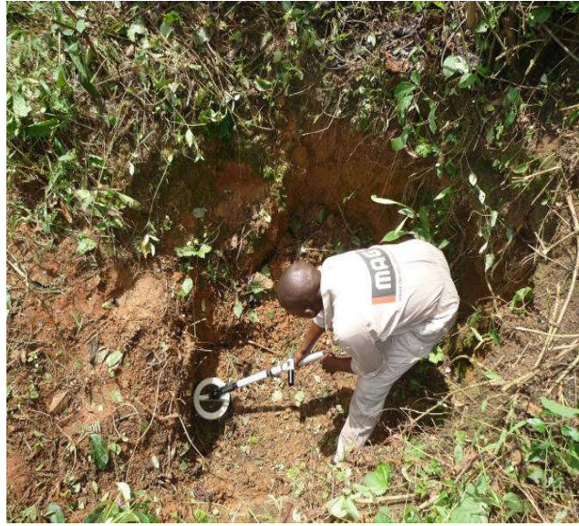
Technical survey to identify the location of an alleged underground unexploded mortar
