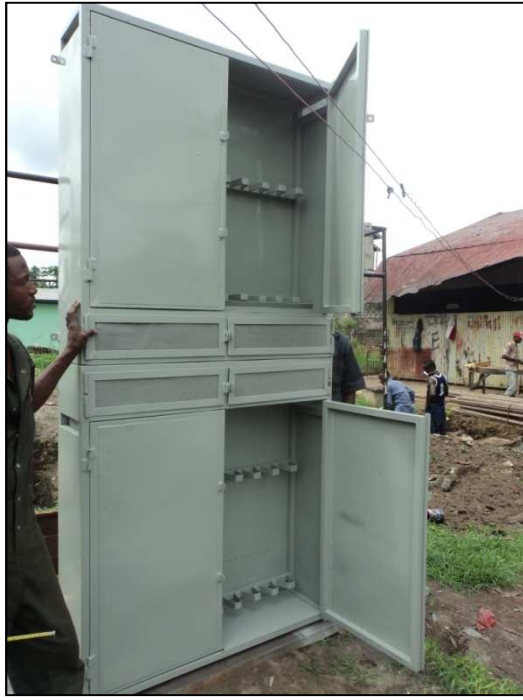
DRC: First prefabricated armoury prototypes
